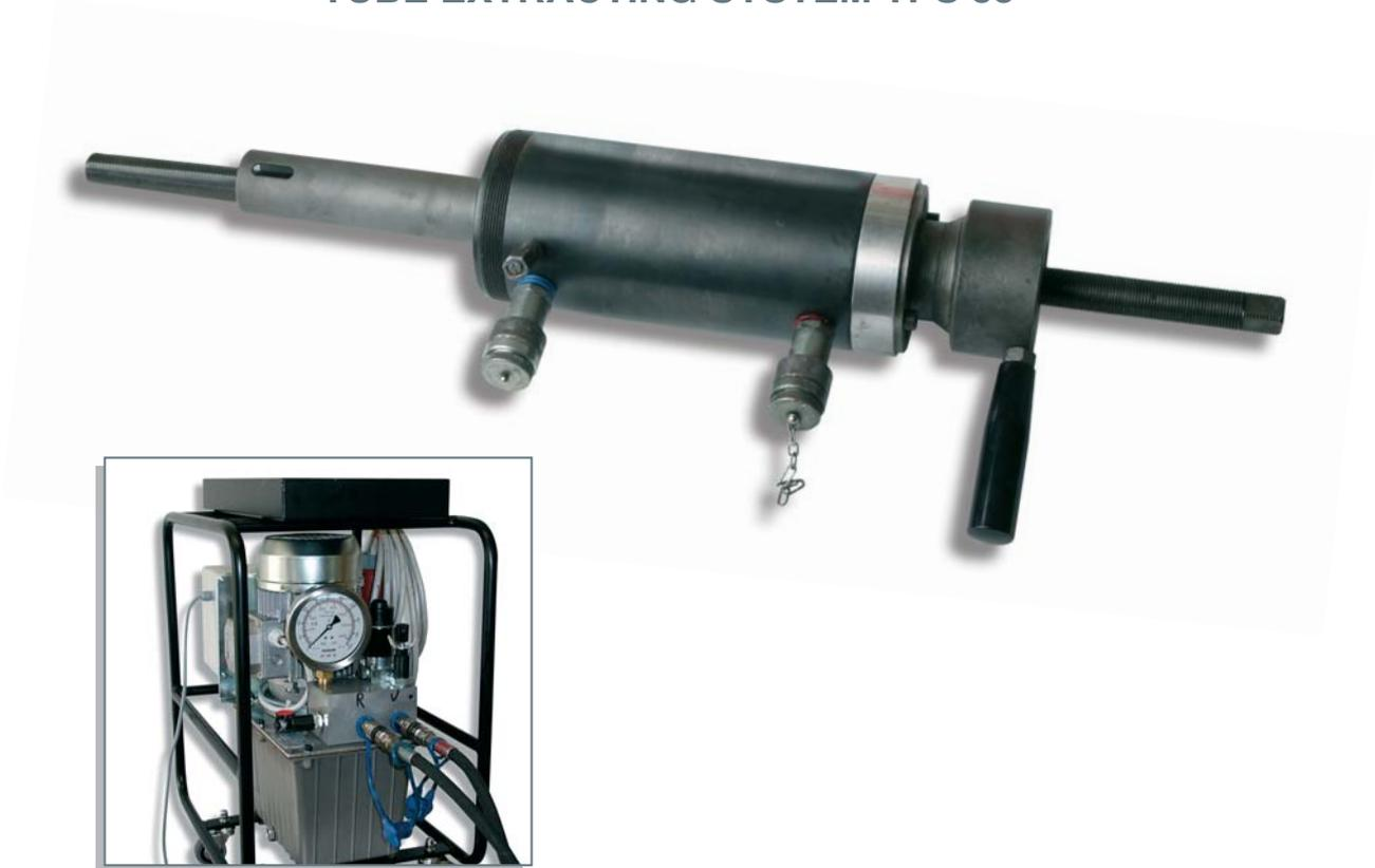
The TPS 55 hydraulic tube extracting machine is a device for **extracting thick-walled tubes** out of the expansion area of tube sheets.
