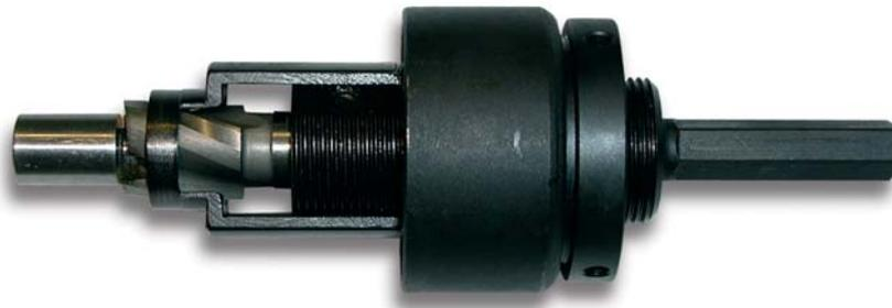
The TF 50 tube end facer is a tool for **manually cutting to length projecting tubes** at the tube sheet and is mounted by means of a Morse taper, a square or a hexagon on a drive machine having a suitable rotary speed and sufficient torque.
